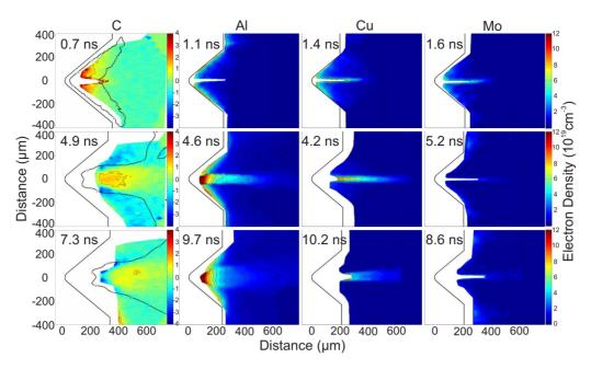
FIG. 2. (Color online) Electron-density maps for C, Al, Cu, and Mo obtained from the interferograms in Fig. 1. Regions in which the density could not be measured due to probe beam refraction are colored white. In the case of carbon the free-electron approximation is computed to be valid in the region to the right of the black line.
