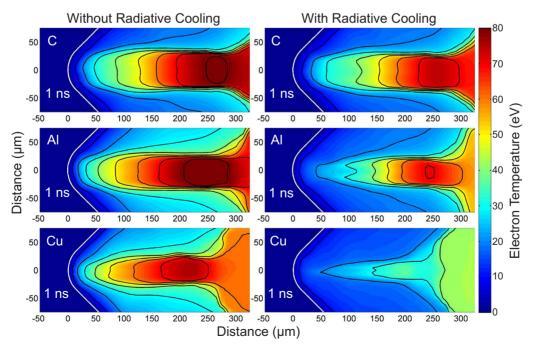
FIG. 6. (Color online) Simulated electron temperature maps for C, Al, and Cu targets at 1 ns into their evolution. Radiation cooling significantly decreases the electron temperature within the higher Z jets.
