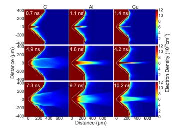
FIG. 3. (Color online) Simulated electron-density maps for C, Al, and Cu plasma jets at different times during the evolution. The irradiation conditions are assumed to be those used to obtain the interferograms in Fig. 1.
