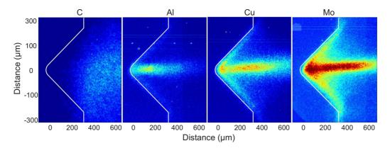
FIG. 5. (Color online) Time-integrated soft-x-ray plasma self-emission images of jets created by laser irradiation of C, Al, Cu, and Mo targets. The amount of radiation emitted by the jet increases with the atomic number of the target material.
