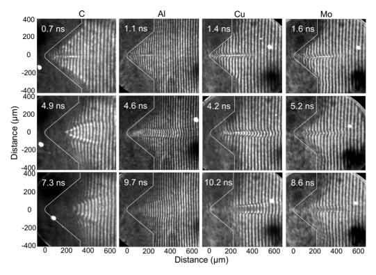
FIG. 1. Sequences of soft-x-ray laser interferograms of plasma jets created by laser irradiation of C, Al, Cu, and Mo targets at intensities of  $\sim 10^{12}$  W cm<sup>-2</sup>. The times are measured with respect to the beginning of the 120 ps laser heating pulse. The position of the target surface is represented by the white line. Jet collimation is observed to increase for the higher Z targets.
