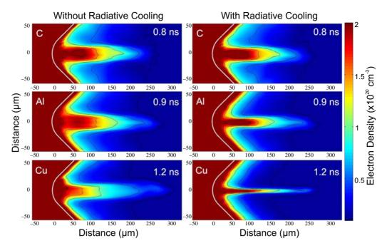
FIG. 4. (Color online) Computed electron-density distribution resulting from simulations with (right column) and without (left column) radiation cooling for C, Al, and Cu plasma jets. The times were selected to allow for jets of similar length. In the absence of radiation cooling a similar degree of collimation is computed for jets of the same length. Radiation cooling increases the collimation of the higher Z jets.
