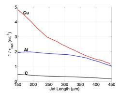
FIG. 7. (Color online) Variation of the radiation cooling rate averaged over the jet volume as the jet evolves reaching different lengths for the C, Al, and Cu plasmas.
